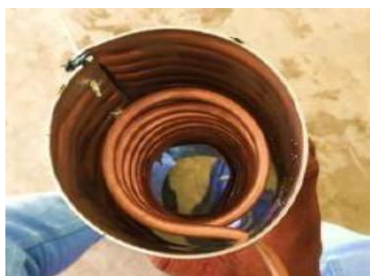
Figure 5: Inner view of the Heat exchanger
