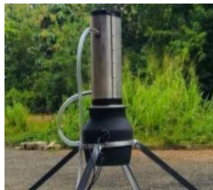
Figure 6: Heating and evaporating unit.
